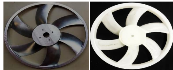
Figure 16. Aluminum reference fan and fan fabricated by centrifugal casting technology (a-reference fan; b-polymer fan).
